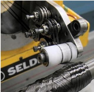
Only the highest grade of pre-pre carbon fibre are used to give sailors the best stiffness-to-weight-spar. The pre-preg carbon tows are UV stabilised to give a guaranteed long life, even in the sunniest of climates. More fibres and less resin, means lighter, stiffer masts.
